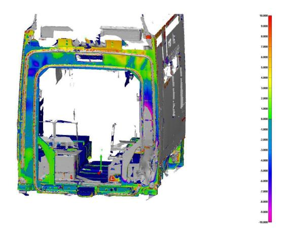
Figure 17: C-Car, A-C Articulation View ±10mm
