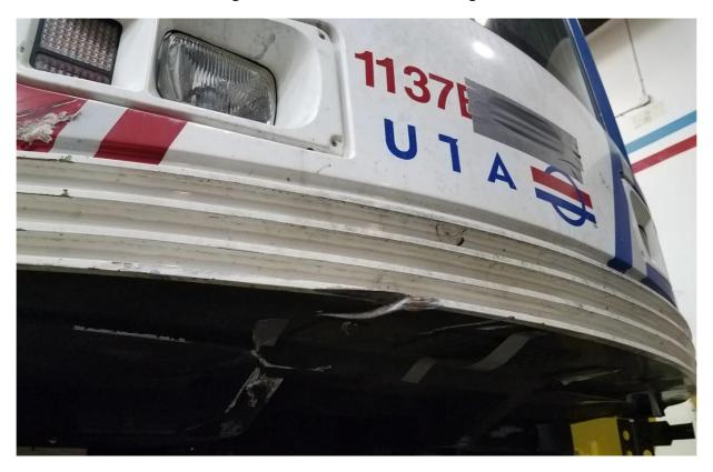
Figure 33: B-Car Anti-Climber Damage
