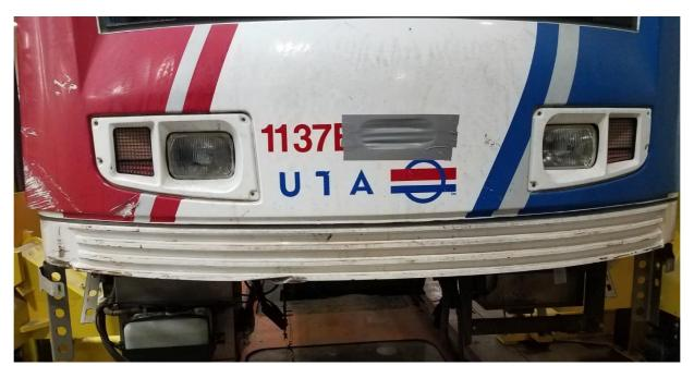
Figure 32: B-Car Anti-Climber Damage
