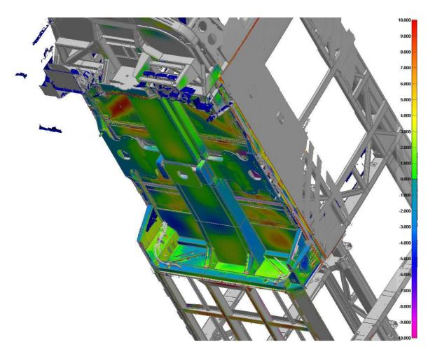
Figure 11: B-Car High Floor Underframe, LH View ±10mm
