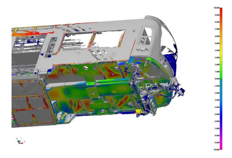
Figure 5: A-Car High Floor Underframe RH ±10mm
