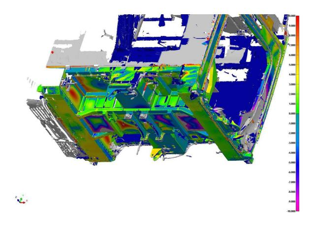
Figure 15: C-Car Non-Impact Side ±10mm
