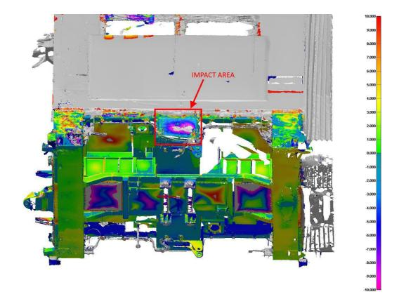
Figure 13: C-Car Impact Side ±10mm
