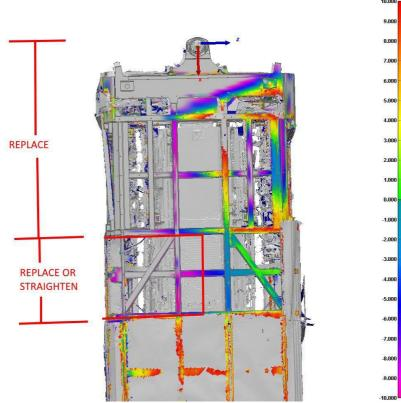
Figure 8: A-Car Low Floor Underframe ±10mm
