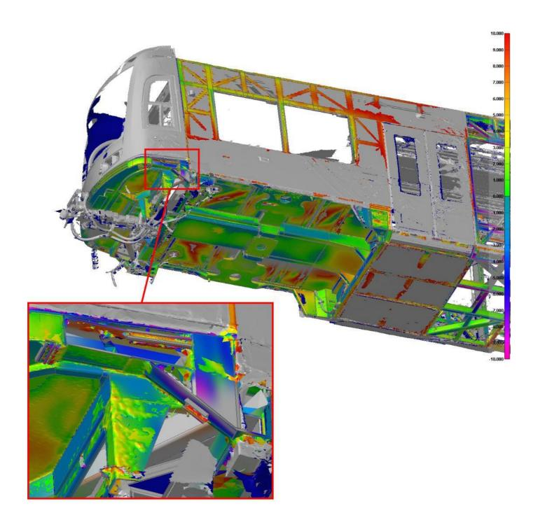
Figure 4: A-Car Cab Underframe LH ±10mm
