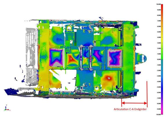
Figure 16: C-Car Underframe ±10mm
