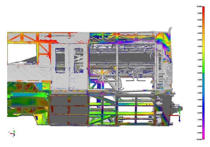
Figure 6: A-Car Low Floor and Sidewall LH ±10mm
