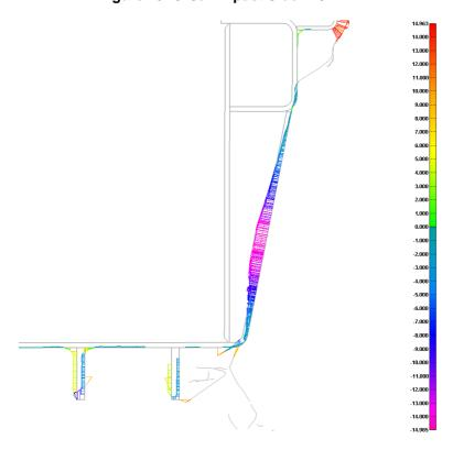
Figure 14: C-Car Impact Cross Section ±15mm
