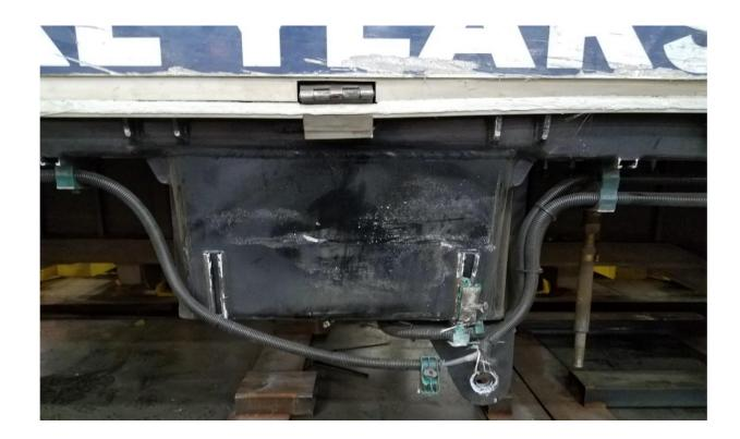
Figure 34: C-Car Impact Side Damage
