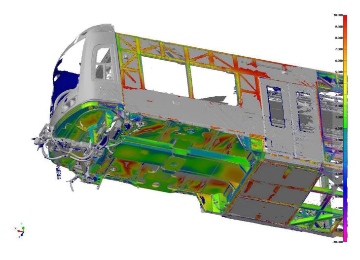
Figure 3: A-Car High Floor Underframe LH ±10mm
