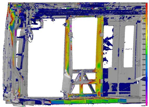
Figure 7: A-Car LH Sidewall Door Portal - Inside View ±10mm
