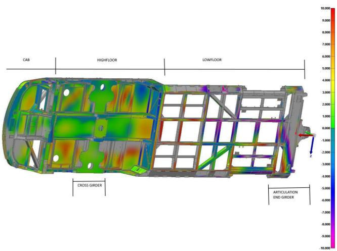
Figure 2: A-Car Underframe Labelled ±10mm Scale
