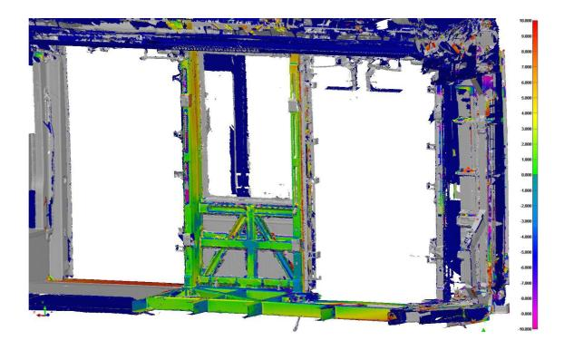
Figure 9: A-Car RH Sidewall Door Portal - Inside View ±10mm
