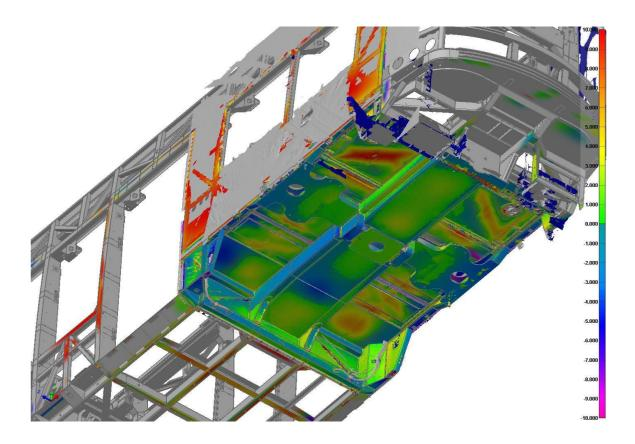
Figure 12: B-Car RH High Floor Underframe ±10mm
